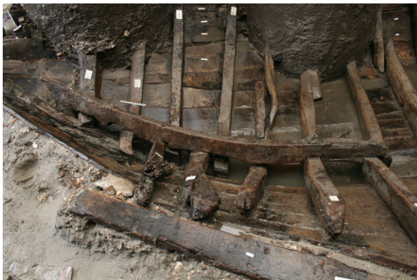
Figure 12. In situ central longitudinal timber on YK 23, either a stemson or sternson; January 2008. (Photo R. Ingram/INA)
