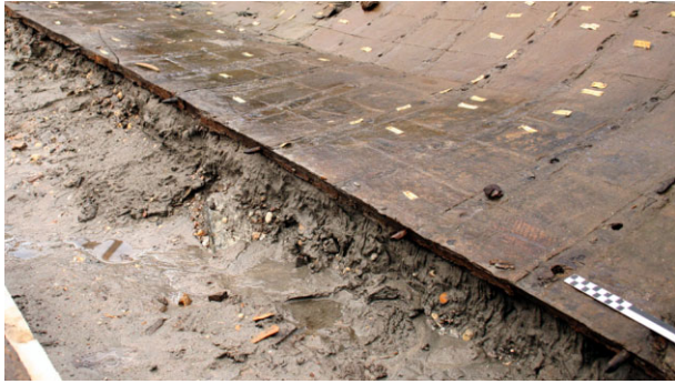
Figure 14. Edge fasteners along exposed plank edge of YK 14; September 2007. (Photo M. Jones/INA)
