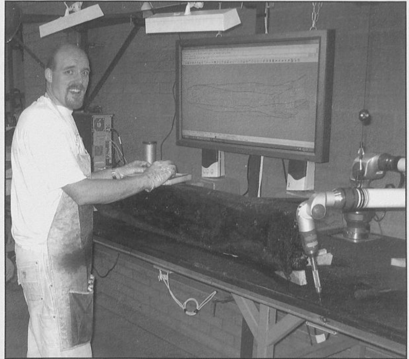
Toby Jones recording ship timbers with a FaroArm three dimensional digitizer at the Newport Medieval Ship Project lab. Photo courtesy of Newport Medieval Ship Project
