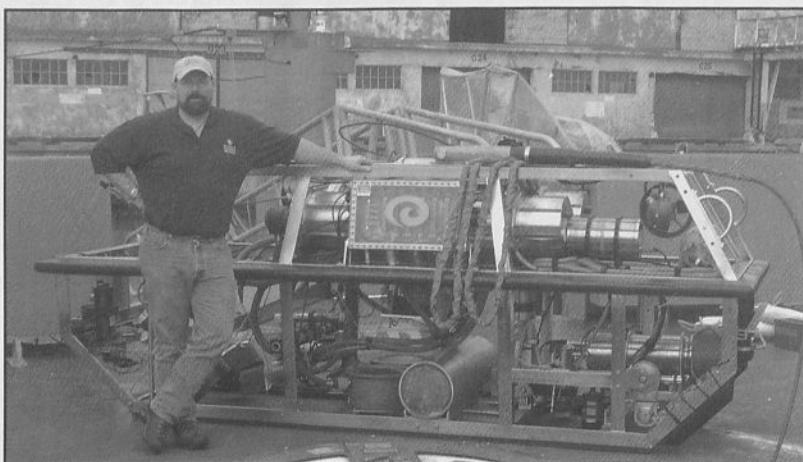
David Robinson with the Institute for Exploration's towed ROV, Argus, which recorded sub-bottom profiles, CTD data, and high-definition video. Photo: Dr. Jack Irion of Minerals Management Service
